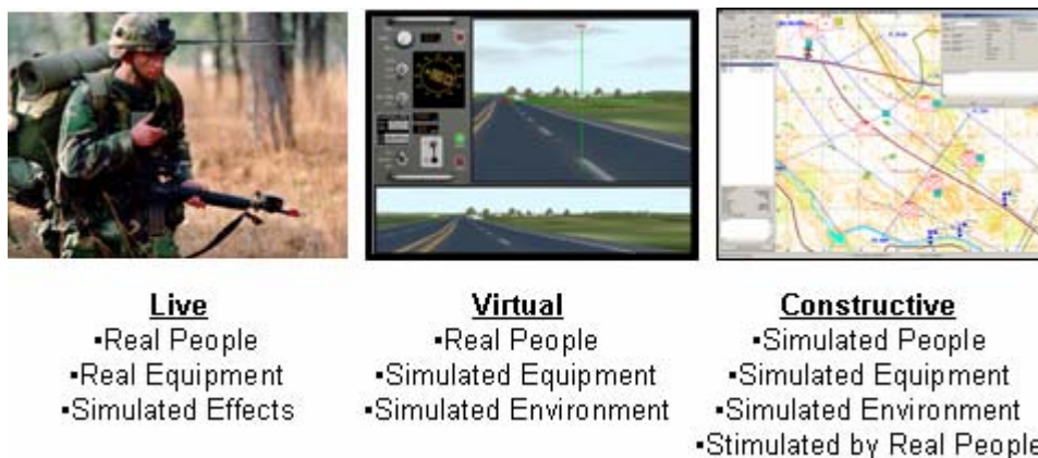
Figure 2: Live, Virtual and Constructive Simulation Definitions.
